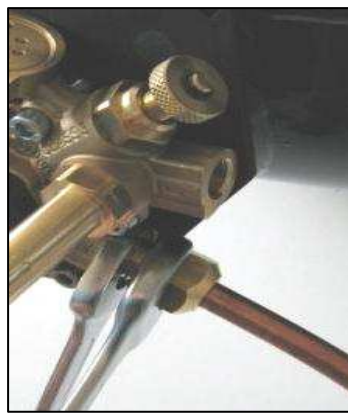
Figure 37: inlet and outlet fittings screwing 0° toroidal tank
