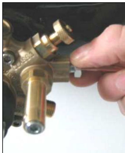
Figure 25: outlet fitting manual connection
