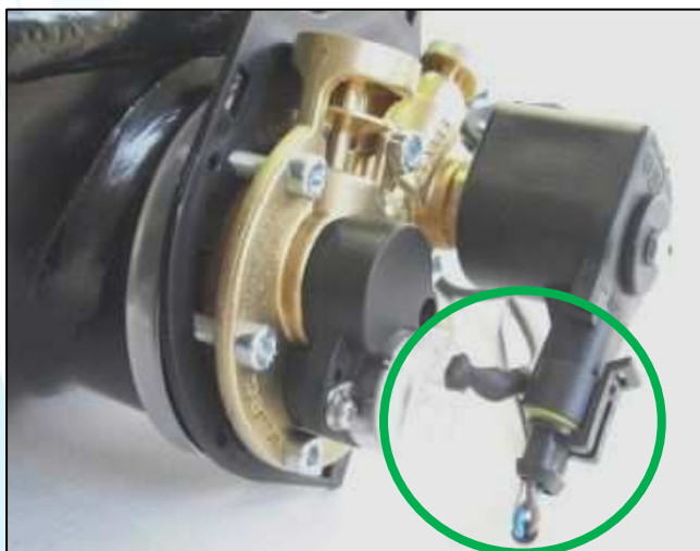
Figure 38: 0° toroidal tank electrical connection and external plastic protection assembly
