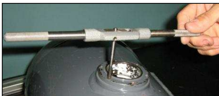
Figure 5: Removing of the paint from the screw threaded holes
