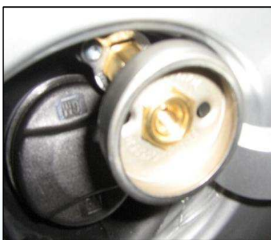
Figure 39: filling point installation
