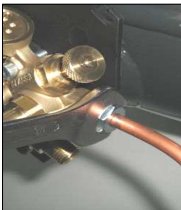
Figure 37: inlet and outlet fittings screwing 0° toroidal tank
